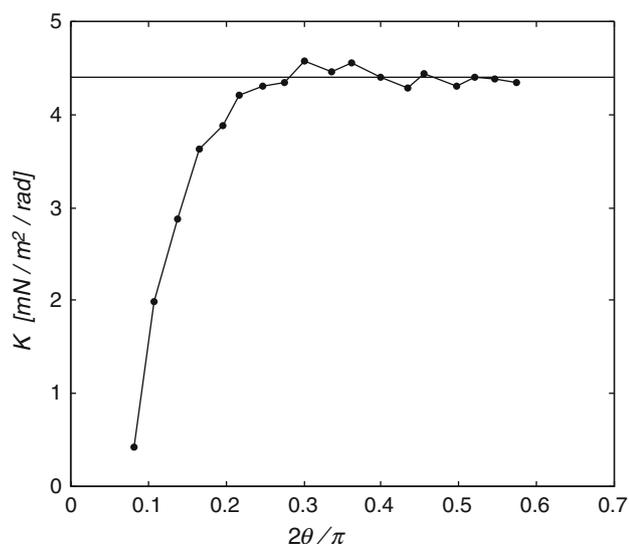
**Fig. 4** Ratio of the torque per unit length of the hinge to the leaflet opening angle,  $K$ , vs. the normalized opening angle. The horizontal reference line indicates the average value,  $K_0$ , of the last nine measured values
