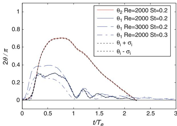
**Fig. 6** Confidence intervals (dotted lines) of the opening angle of leaflet #1 (blue line) and #2 (red line) for non-symmetric leaflets ( $\varepsilon = 0.5$ ). Dashed and dash/dotted lines indicate the angle of the short leaflet at  $Re = 3,000$ ,  $St = 0.2$  and  $Re = 2,000$ ,  $St = 0.3$ , respectively
