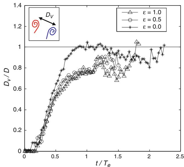
**Fig. 14** Non-dimensional distance between vortices vs. non-dimensional time in the different leaflet configurations
