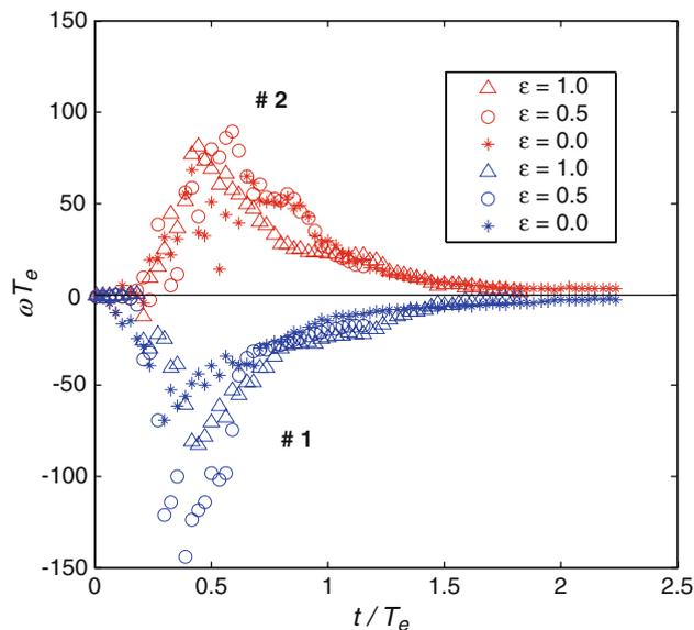
**Fig. 16** Non-dimensional average vorticity of vortex #1 (blue symbols) and #2 (red symbols) as a function of the non-dimensional time in the tested leaflet configurations
