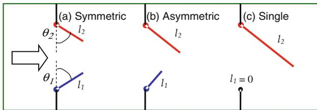
**Fig. 2** The three tested leaflet configurations on the test plane with leaflet aperture angles
