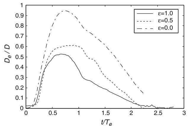
**Fig. 7** Effective leaflet aperture,  $D_e$ , non-dimensionalized by the orifice width as a function of the non-dimensional time
