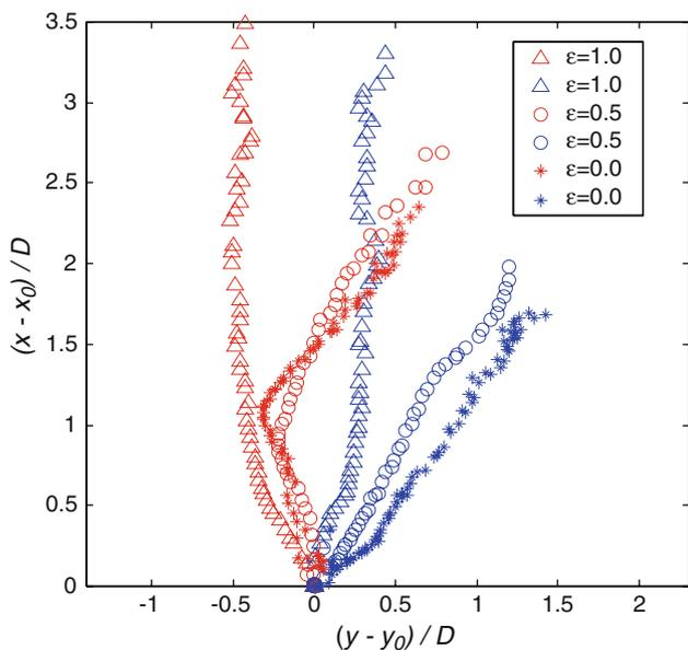
**Fig. 11** Trajectories of the vortex #1 (blue symbols) and #2 (red symbols) for the tested leaflet configurations [the coordinates refer to the initial position of the vortices ( $x_0; y_0$ )]
