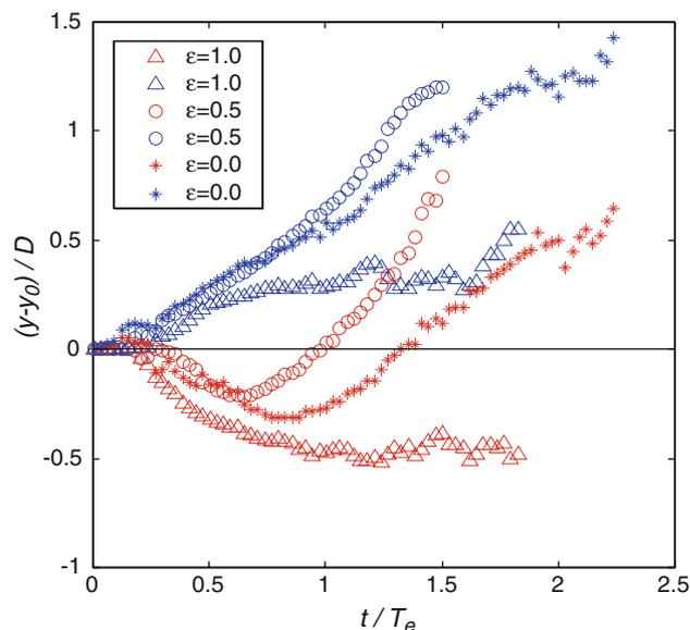
**Fig. 13** Spanwise position of the vortex #1 (blue symbols) and #2 (red symbols), as a function of time for the tested leaflet configurations
