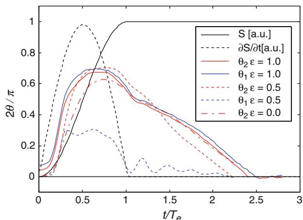
**Fig. 5** Piston position and velocity in time (arbitrary vertical units) with leaflet angular positions in the different configurations. Left leaflets are indicated in red and right leaflets in blue
