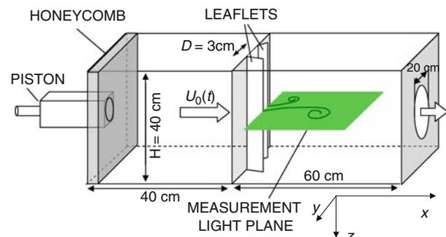
**Fig. 1** The moving leaflet jet apparatus with coordinate system
