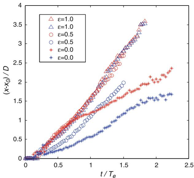
**Fig. 12** Downstream distance travelled by the vortex #1 (blue symbols) and #2 (red symbols), as a function of time for the tested leaflet configurations
