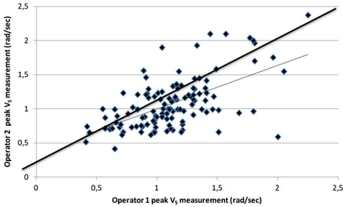
**Fig. 3.** Scattergram plot of  $V_S$  values for Operators 1 and 2. The solid thicker line indicates the quadrant bisector line ( $y = x$ ), while the solid thinner line is the linear regression of observed values ( $y = 0.639x + 0.355$ ).
