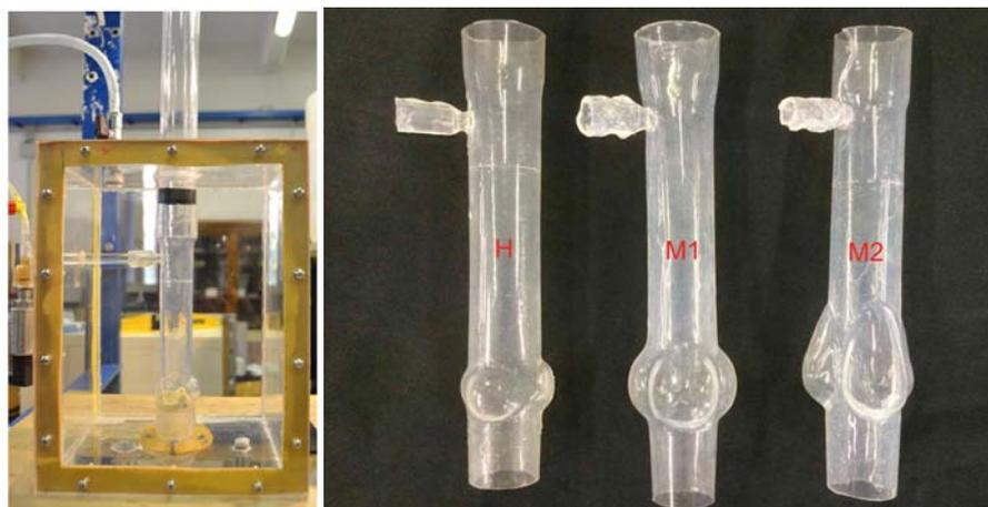
**Fig. 2** On the left: a picture of the aortic chamber. On the right: the model aortas used during the experiments; healthy (H), M1 and M2 from left to right.
